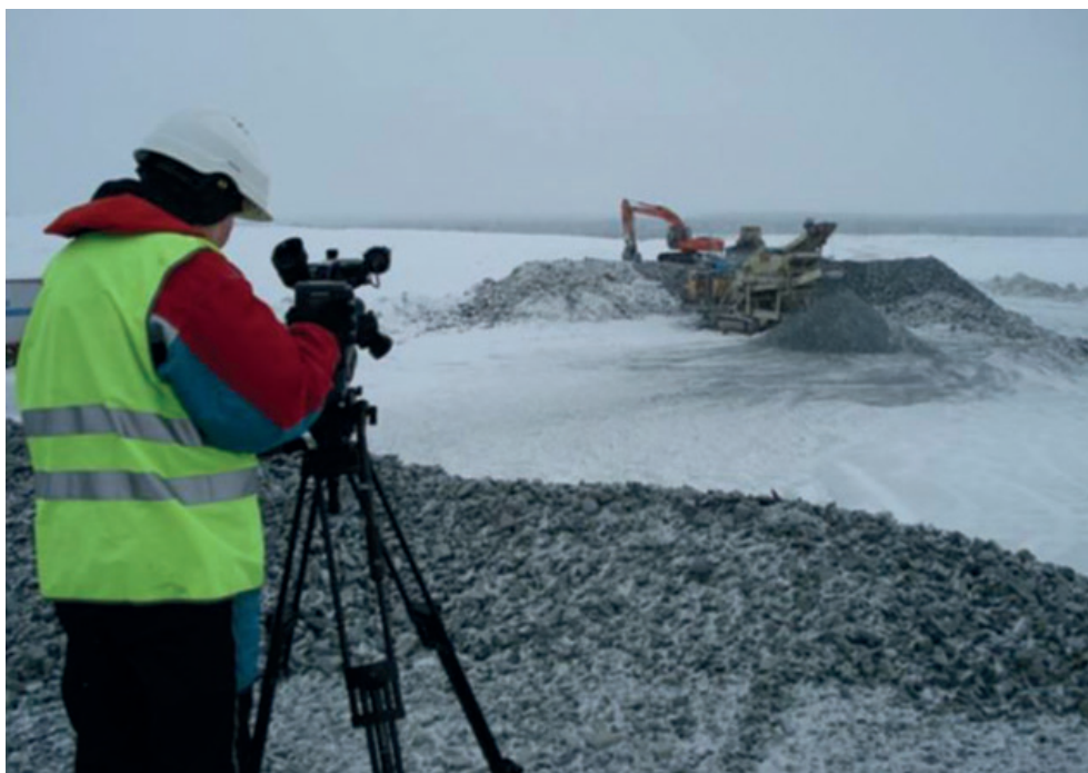
Figure 22. Noise measurement at the Kittilä Mine. (Photo: Agnico-Eagle Mines Ltd.)
