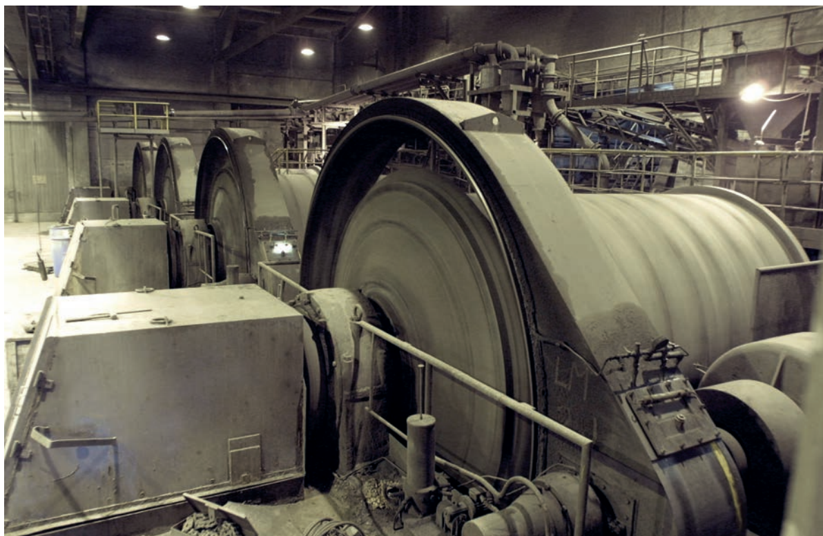
Figure 7. Grinding mills at the Pyhäsalmi mine. (Photo: Pyhäsalmi Mine Oy)
