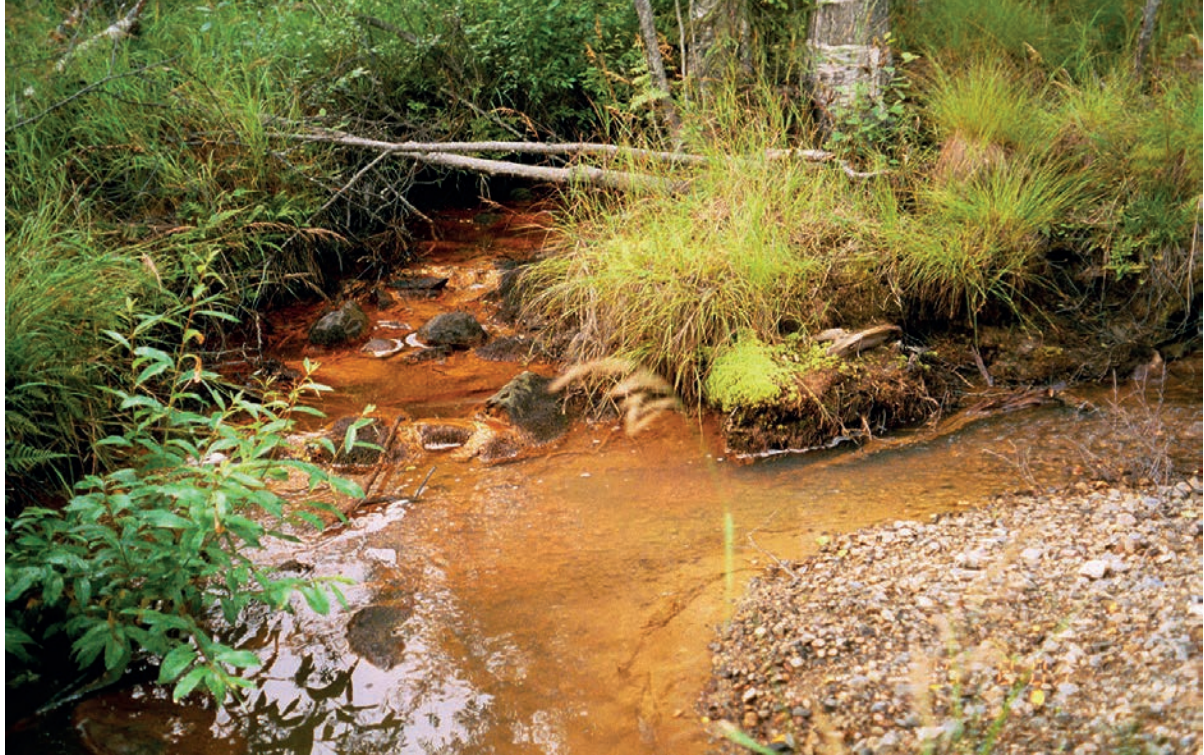
Figure 24. Acid seepage containing iron precipitate (reddish brown) and metals, discharging from a waste rock pile containing oxidising iron sulphides. (Photo M.L. Räisänen)
