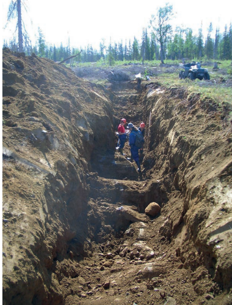
Figure 2. Left: Sampling for MMI in Lapland. Right: Survey trench dug by excavator for bedrock and soil survey and heavy mineral sampling. Studies of the area were continued using in situ sampling of weathered rock and till and drilling. (Photos: Janne Hokka)
