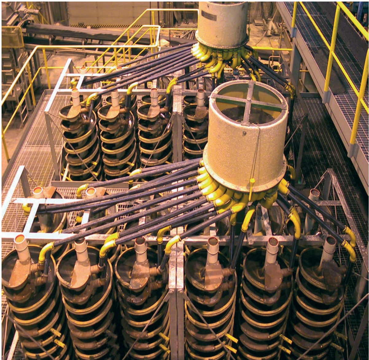
Figure 10. Spiral classifiers used in gravity separation at the Kemi mine. (Photo: Outokumpu Oy)
